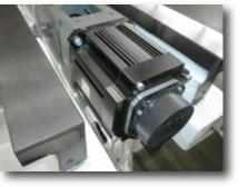
16mm fine pitch ballscrews in combination with 67 million pulse encoder technology provide a new degree of contouring accuracy - at least 4x smoother surface finishes are achieved as a result of this technology.
